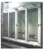
Procedure of classification: DIN EN 12207:2000. Windows and doors. Air permeability. Classification. DIN EN 12208:2000. Windows and doors. Watertightness. Classification. DIN EN 12210:2000. Windows and doors. Resistance to wind load. Classification. DIN EN 12210/AC:2002. Windows and doors. Resistance to wind load. Classification.
