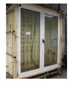
Procedure of classification: DIN EN 12207:2000. Windows and doors. Air permeability. Classification. DIN EN 12208:2000. Windows and doors. Watertightness. Classification. DIN EN 12210:2000. Windows and doors. Resistance to wind load. Classification. DIN EN 12210/AC:2002. Windows and doors. Resistance to wind load. Classification.
