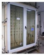
Procedure of classification: DIN EN 12207:2000. Windows and doors. Air permeability. Classification. DIN EN 12208:2000. Windows and doors. Watertightness. Classification. DIN EN 12210:2000. Windows and doors. Resistance to wind load. Classification. DIN EN 12210/AC:2002. Windows and
